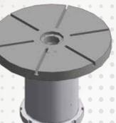
Utilizes an integrated spindle sleeve structure to prevent precision loss due to table accuracy deviations. The extended support and preloaded positioning design enhance rigidity and minimize vibration, improving machining precision.
