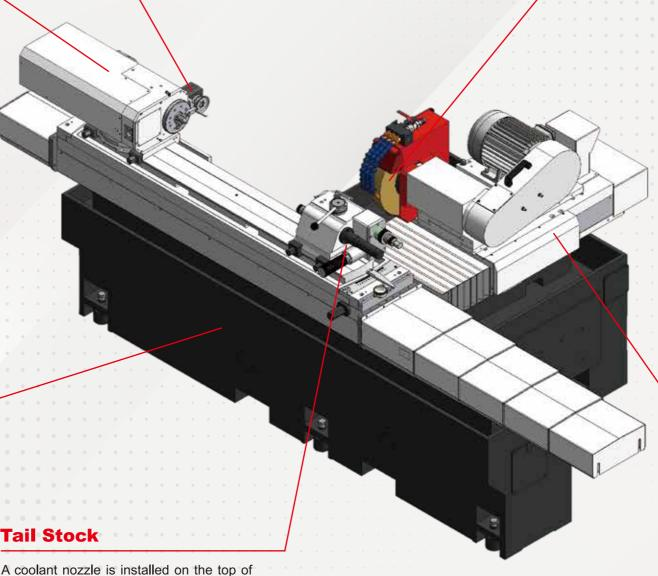
the tailstock for cooling the center tip. An
