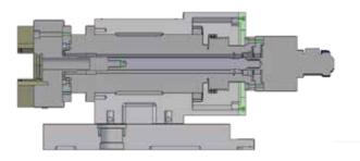
We Use the original C axis to drive and carry BT spindle. The spindle head design places the center of gravity at the rear portion to help balancing the whole spindle mechanism to increase spindle accuracy and loading capacity.
