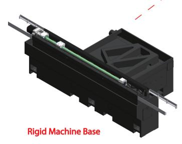
The machine based is designed to ensure the table is fully supported on both ends. The heavily ribbed box-type base is made of Meehanite casting, providing excellent rigidity and stability of the machine. The features include increasing 33% of the base span which strengthen the center of gravity support for workpiece grinding.
