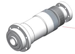
Complete one piece cartridge spindle can avoid the eccentricity of spindle housing and reduces the thermal growth, thus increase spindle life.
