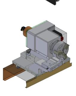
Low-gravity base structure, with slant bed design
