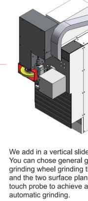
We add in a vertical slide mechanical structure. You can chose general grinding wheel or diamond grinding wheel grinding the end face of the spindle and the two surface planes of the locating key with touch probe to achieve automatic positioning and automatic grinding.
